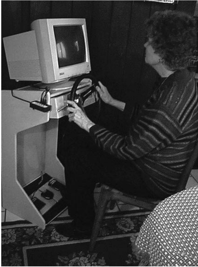
Figure 43-7. Elemental Driving Simulator (EDS) standard model. An IBM-compatible personal computer (not shown) controls a dynamic display of a schematic roadway and peripheral stimuli. The patient controls the lateral position of the “car” using the steering wheel and uses the turn signal to make responses. For hemiparetics, the foot pedals are used for responding.
