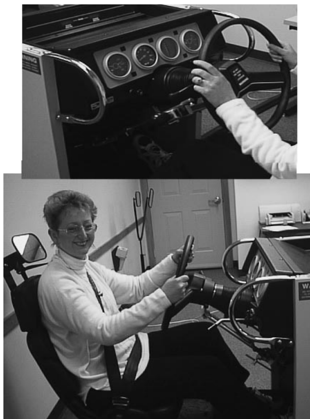
Figure 43-11. Doron Driver Analyzer at the Easter Seals Mobility Center. When performing the simulation, the patient would be viewing a video projected on a large screen directly ahead. The console is physically realistic; however, the task is not interactive (i.e., nothing that the patient does changes the display).
