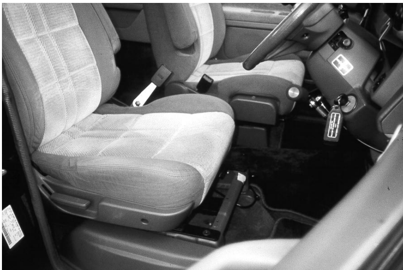
Figure 43-5. The driver's seat was substantially repositioned to the rear to enable Patient A to sit in it. A seat belt extension, which can be seen between both seats, enables him to locate and engage the seat belt.
