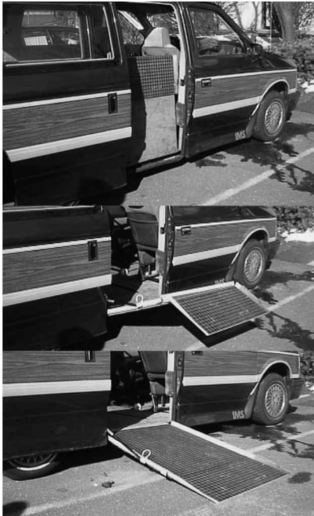
Figure 43-13. Adapted van at the Easter Seal Mobility Center. The floor has been lowered by 10 inches on this van. A side-mounted hoist installed in a van allows self-loading and driving from a wheelchair. Top. The door opens by remote-controlled switch. Middle. The hoist lowers automatically. Bottom. Hoist in wheelchair loading/unloading position.
