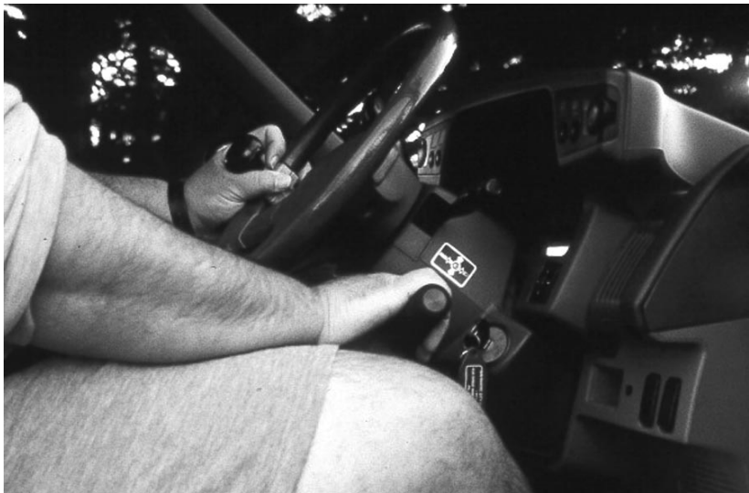
Figure 43-3. Patient A demonstrates hand controls and steering wheel spinner. Even in the most ideal vehicle, space for equipment was limited.
